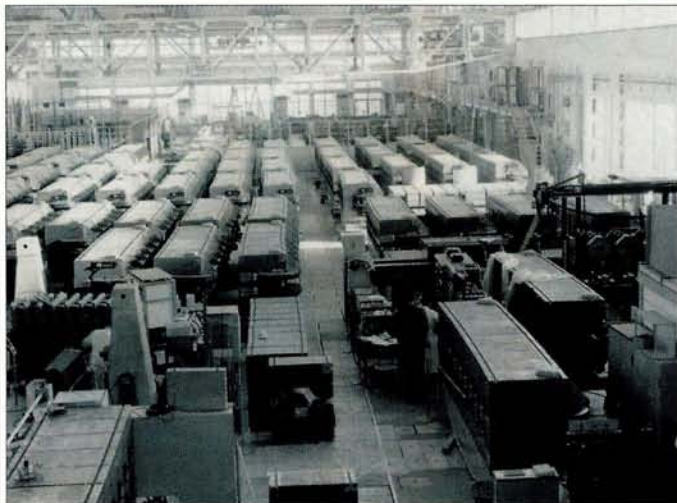
Completed magnets in the South Hall wait to be installed in the PS ring in October 1958 – a view comparable to that of today’s stock of “cold masses” for the Large Hadron Collider (p33).
