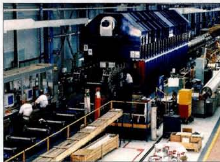
One cold mass during welding, with another waiting behind the press, at Alstom in Belfort, France. The two welders controlling the welding remotely can be seen on the left.
