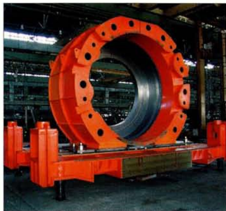
A test assembly of the table and shielding cylinder for the CMS at the Iranian manufacturers HEPCO. (Photo: T de Visser.)
