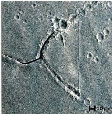
Fig. 3. This graphic shows surface damage associated with grain boundaries, perhaps as a result of localized ohmic heating. (S Harvey, SLAC.)
