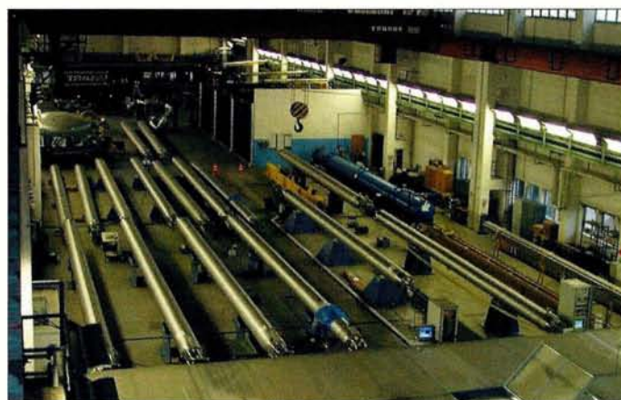
Fig. 7. The stock of finished and almost finished cold masses at the Babcock Noell Nuclear workshop in Zeitz.
