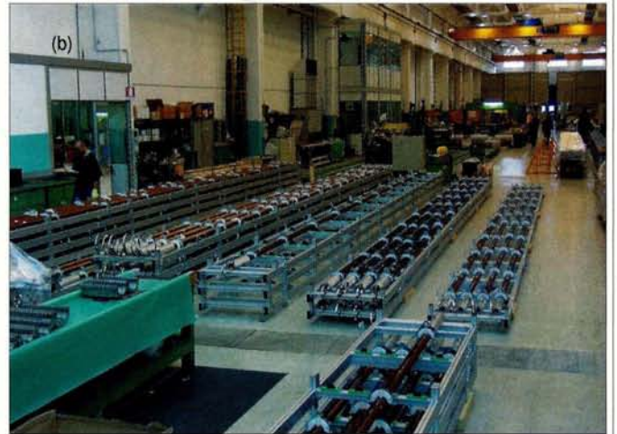
Fig. 2. (a) The actual and expected learning curves for the manufacture of a complete dipole collared coil at Babcock Noell Nuclear in Würzburg, Germany. Values are normalized to the final target. (b) Coils waiting for pole assembly at Ansaldo in Genova, Italy.
