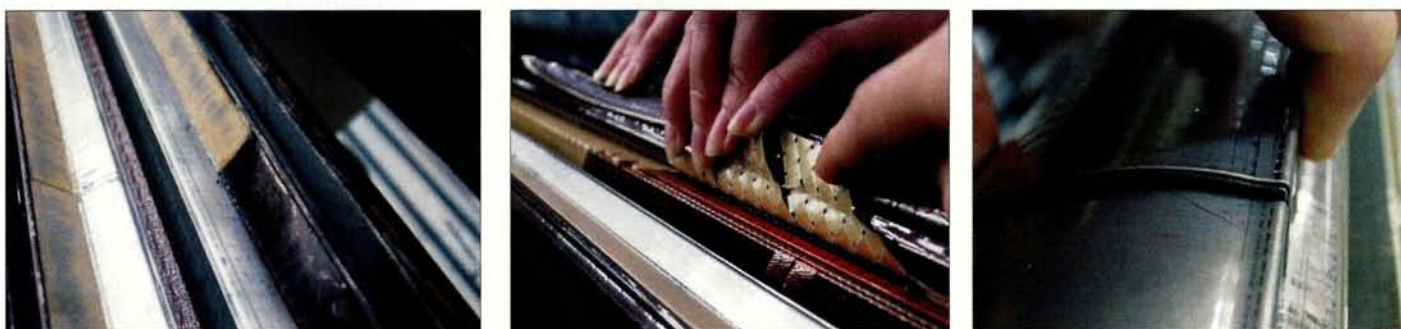
Fig. 5. In room-temperature measurements of the magnetic field of more than 220 magnets at the main dipole manufacturers, three cases of bad assembly procedures have been found and cured (by November 2003): a missing shim of 0.8 mm thickness (left), a coil presenting some turns not glued to the inner layer, leading to cable displacements of 1 mm (centre), and a double coil-protection sheet of 0.5 mm thickness (right).
